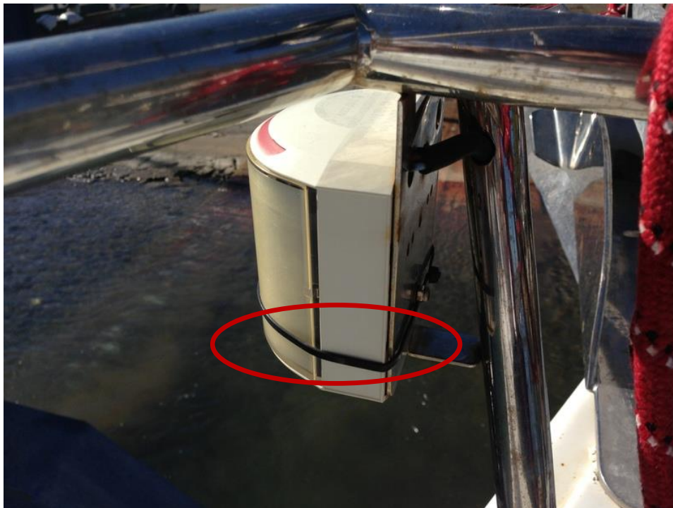
Port navigation light was supported by a plastic strip.
