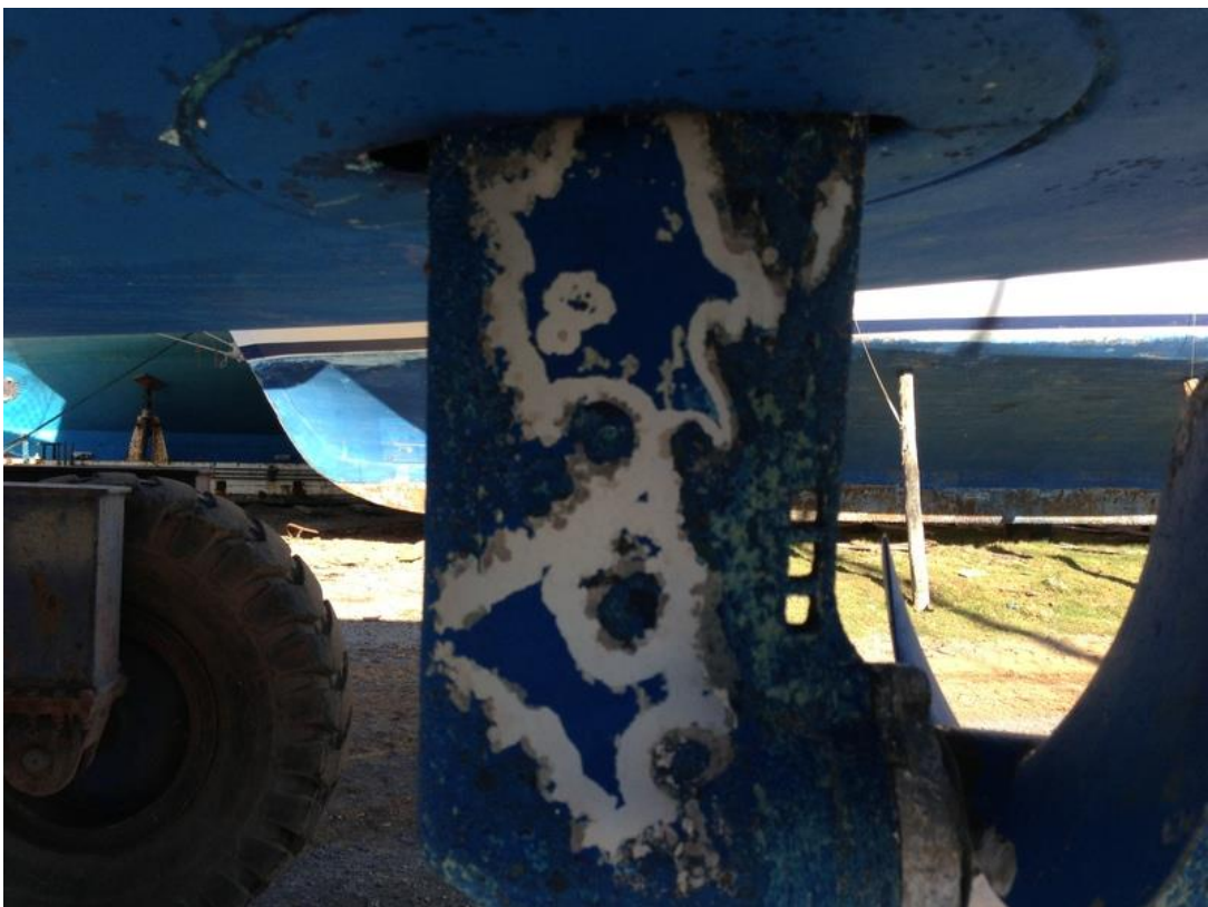
Sail-drive transmission system and three blade fixed propeller has not corrosion but they were painted with dark blue antifouling. Applying this grp antifouling is not acceptable for engine manufacturer. These must be painted by special metal antifouling.
