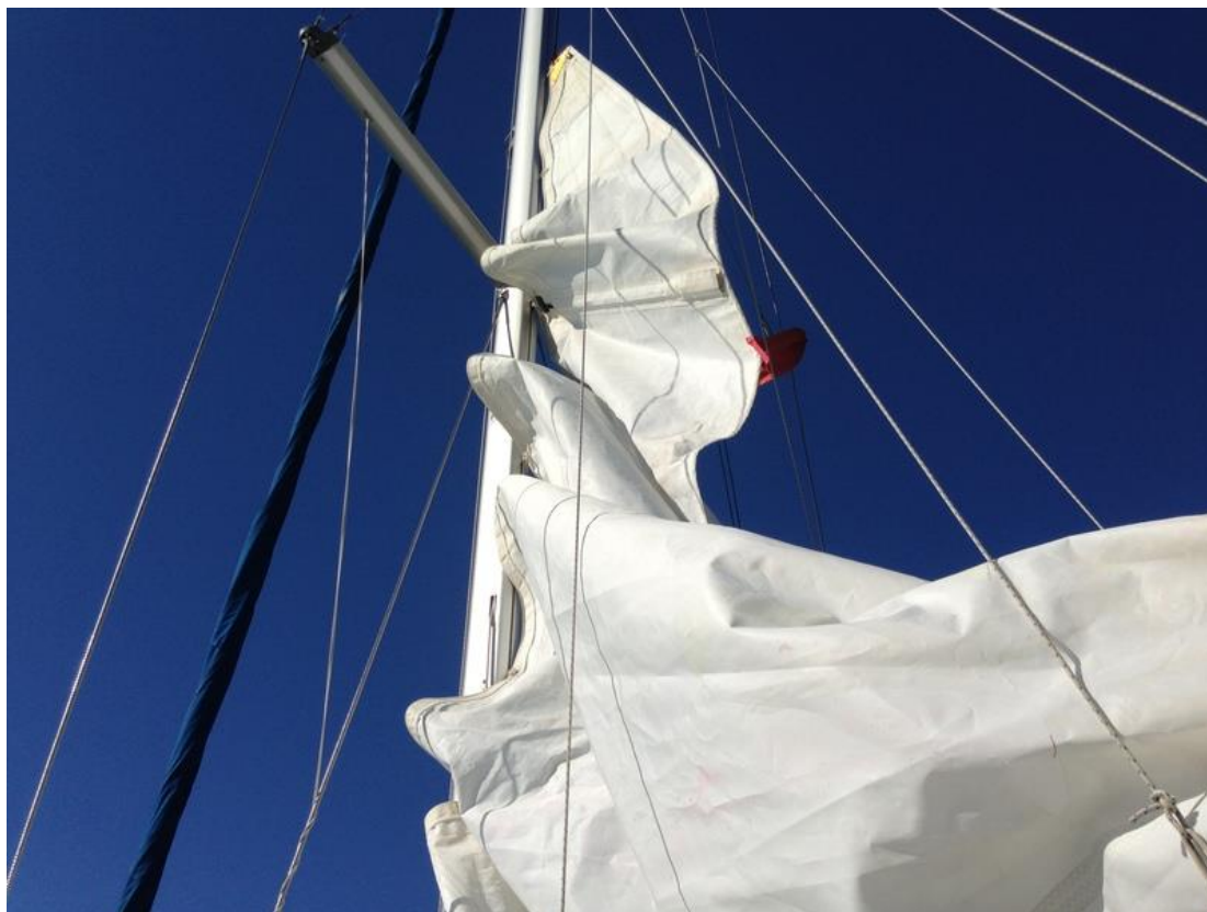
Mainsail stayed above the level of spreader.
