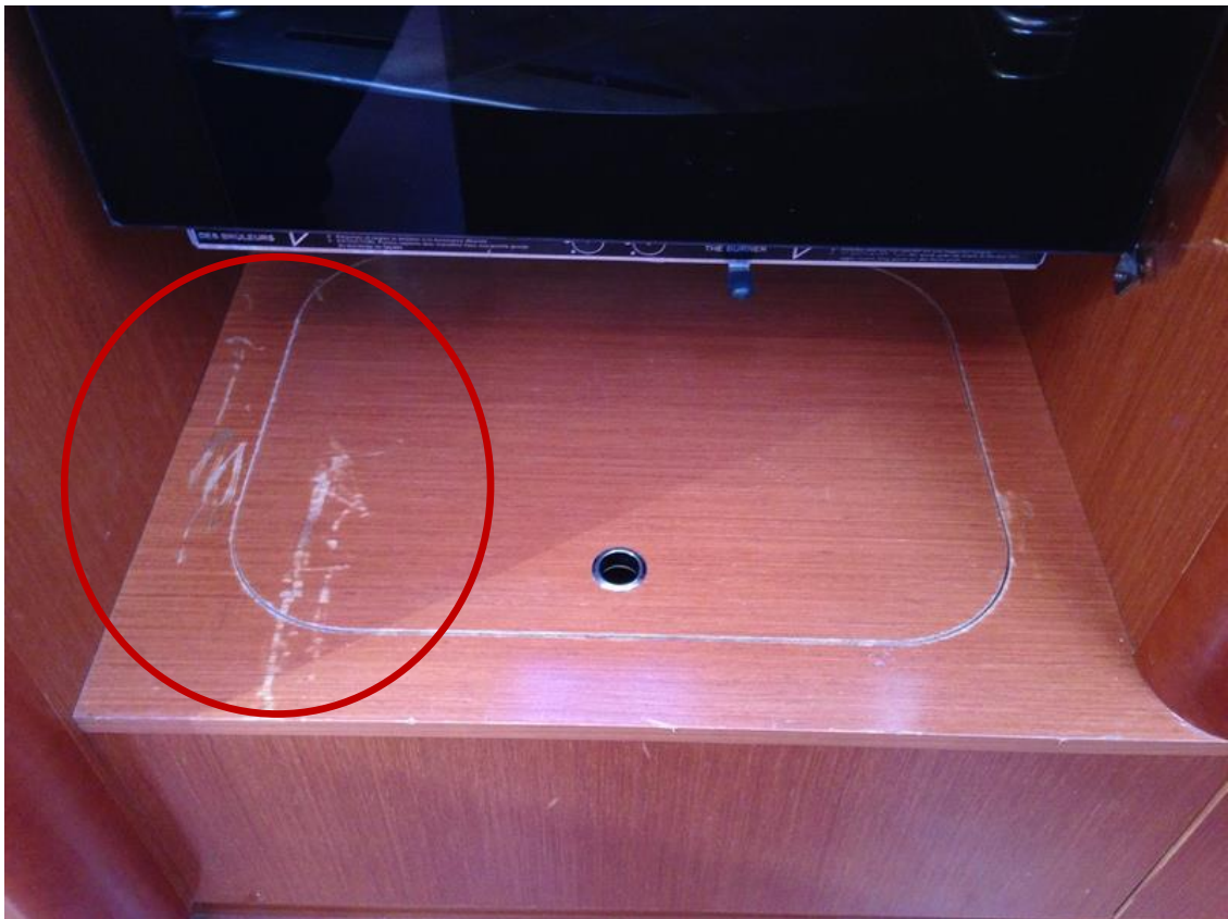
Cosmetic defects on saloon.
