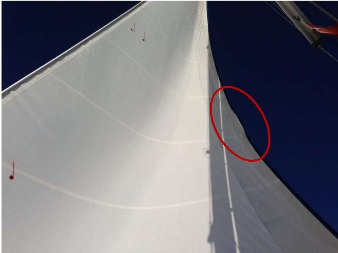
Leech side of genoa, uv protection cushion started tearing.
