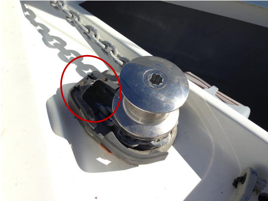
Chain cover of windlass was broken.
