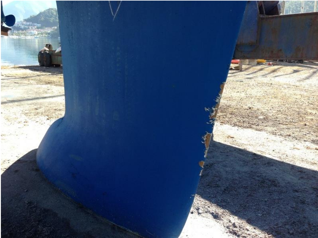
Bottom and bow side of the keel has some damages.
