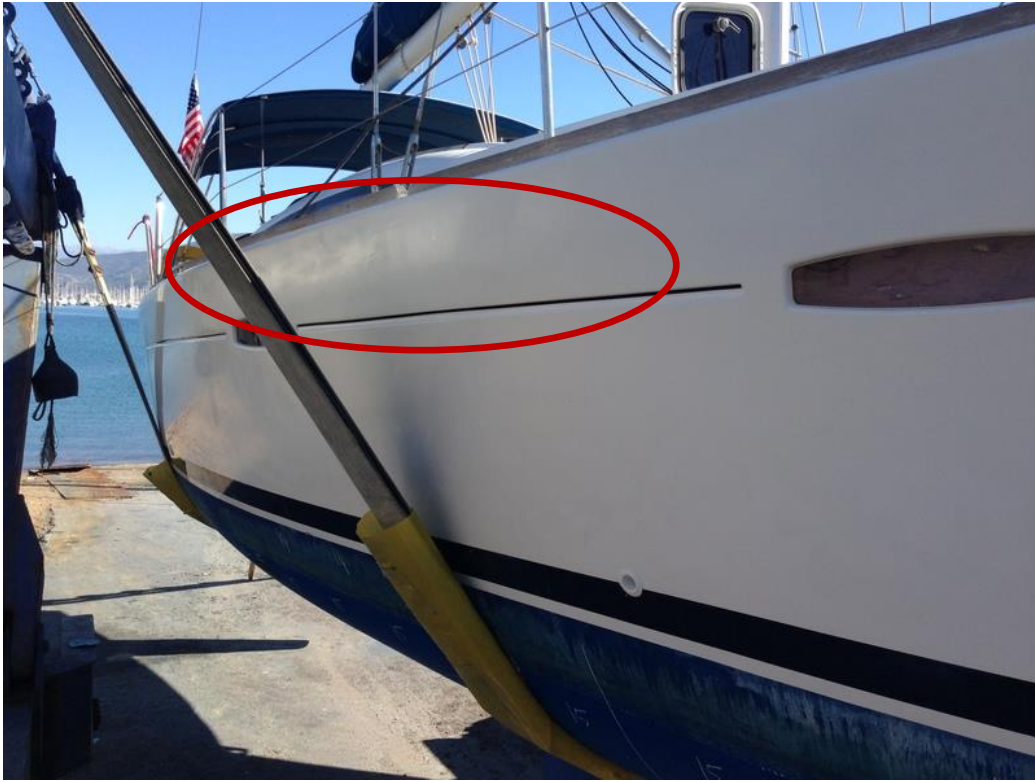
Topside white gelcoat surfaces are not shining enough. This was and then protection polish can be done before the next summer session.
