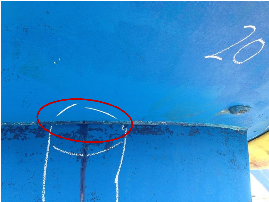
A hole type detachment on sealing between grp hull and keel.
